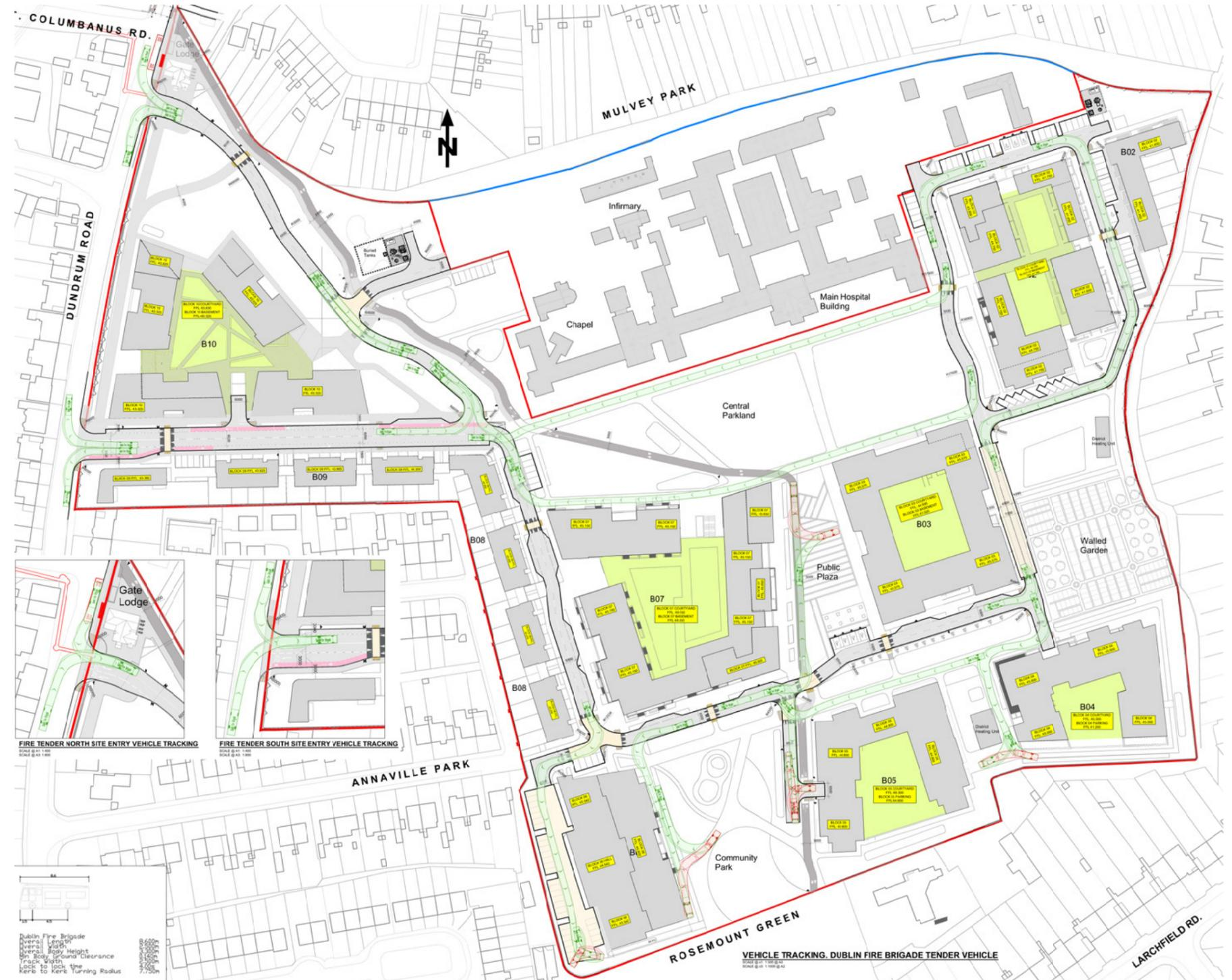
Figure 18 - Proposed fire tender access drawing (See drawing DCD-BMD-00-00-DR-C-1005 by BMCE submitted as part of this planning application for further detail)
